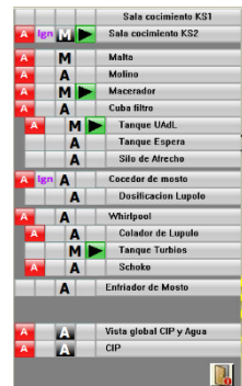
Figure 7 Hierarchical Menu structure with status indicators
