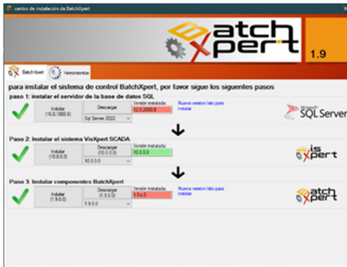
Figure 11 System Installation is guided by Installation tools
